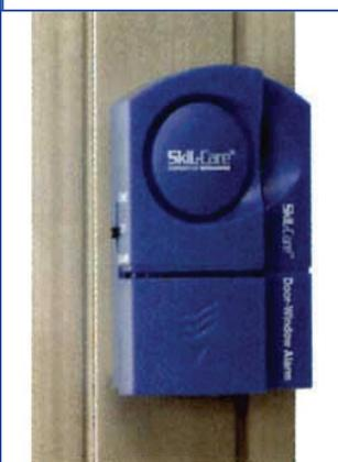
These easy-to-install **Door/Window Alarms** are designed to help minimize the dangers of wandering associated with Alzheimer's. The alarm sounds a warning letting you know that an exit door or window has been opened. The alarm has a three-positions switch for selecting between off, a chime sound and an alarm. Once the door or window is closed, you can reset the alarm. The vendor says that door/window alarm installs easily in seconds with adhesive
